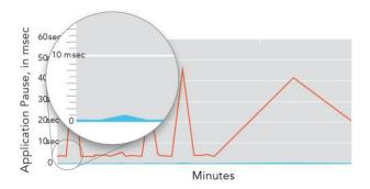
Azul Platform Prime reduces peak pauses from over 40 seconds to under 5 milliseconds
